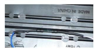
Underside of an HO track. Notice placement of reed switch is in between the rail and the slot. You may use hot glue to hold it in place.
