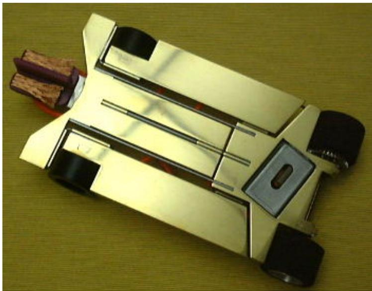
This set up is most effective if the chassis has a degree of "plumber" movement. The more 'weight' or force on the guide under braking and during cornering, the harder it is for the guide to come out of the slot. "Plumber" movement allows the transfer of weight to the front of the chassis under braking, by allowing the rear of the pans and body to lift slightly. This is achieved through upwards hinging, to assist the weight transfer.
